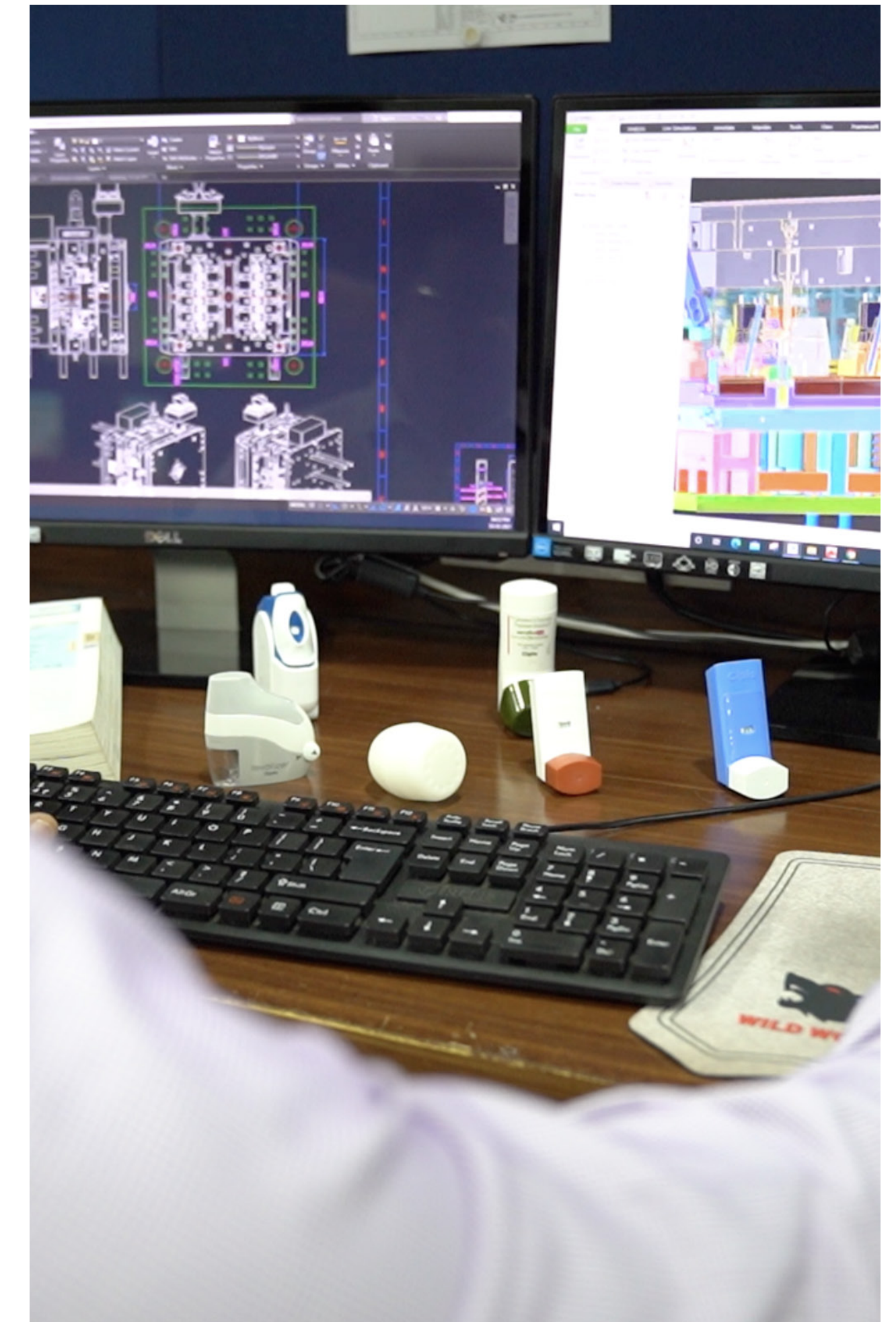
Engineer working on a new mould design.
