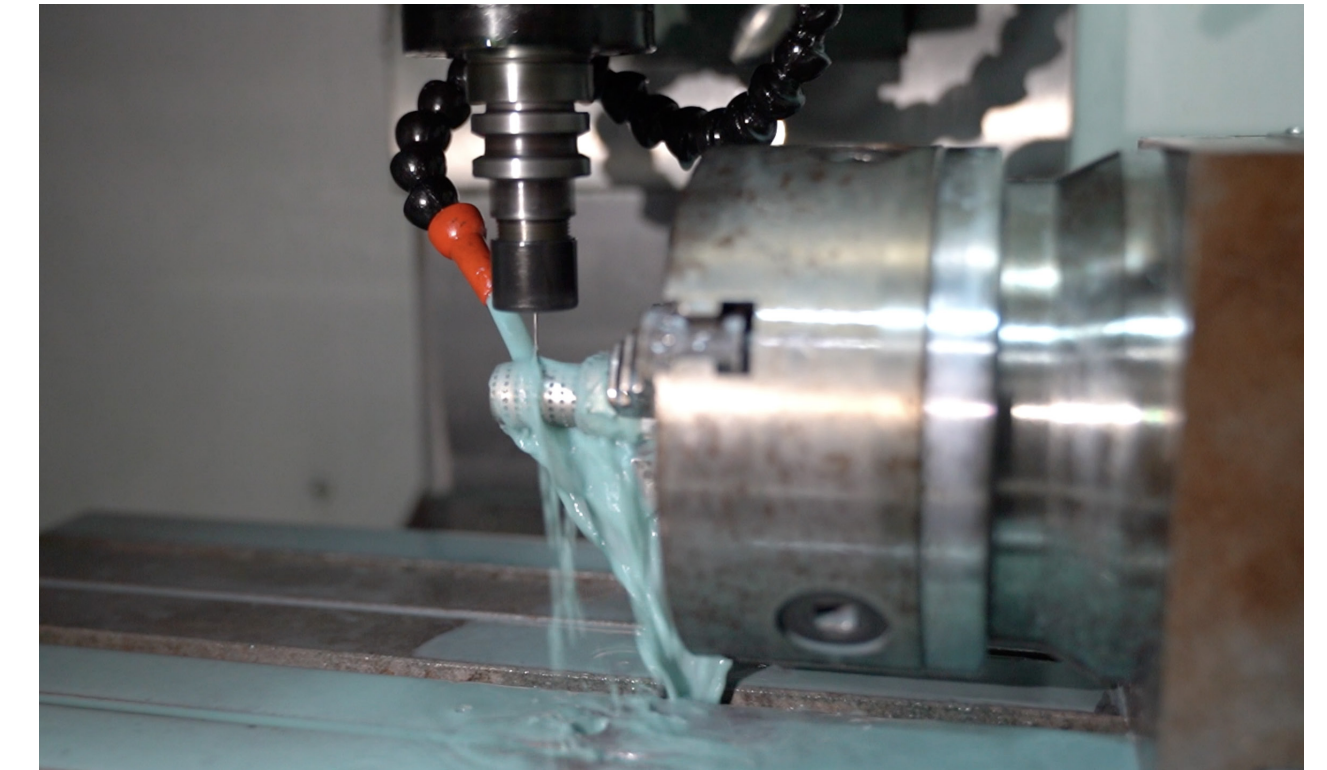
Machining of a part using a fourth axis attachment.
